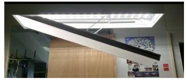
After release the locking hook, the inner box with mounting membrane will swing down and stay in half-open position by two spring hooks. LED tapes on outer frame are accessible.
